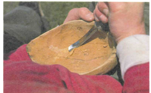
Using a crooked knife to gouge out a bowl.
